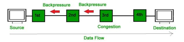
In above diagram the 3rd node is congested and stops receiving packets as a result 2nd node may be get congested due to slowing down of the output data flow. Similarly 1st node may get congested and inform the source to slow down.
